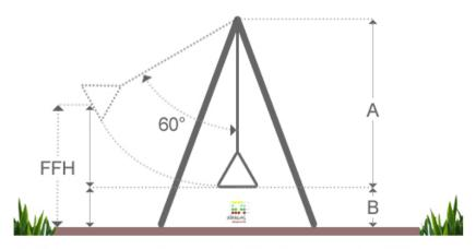
The free fall height is calculated from the centre of the stationary seat surface at 60 degrees. To work this out divide the length of the chain by 2 then add the distance from the seat to the ground. The image above demonstrates this.
